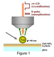
wave (cw) laser diode ( $\lambda$ =830 nm) was used to erase the amorphous region by thermal annealing crystallization.
